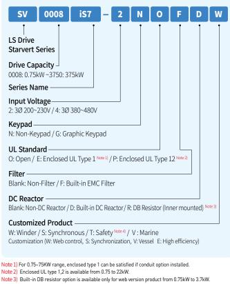
(12.3) Built-in DB resistor of IS7 porduct is available only for web version product from 0.75kW to 3.7kV DB resistor of IS7 porduct is the option of WEB product. Applicable capacity is from 0.75 to 375 kW of IS7 porducts.
